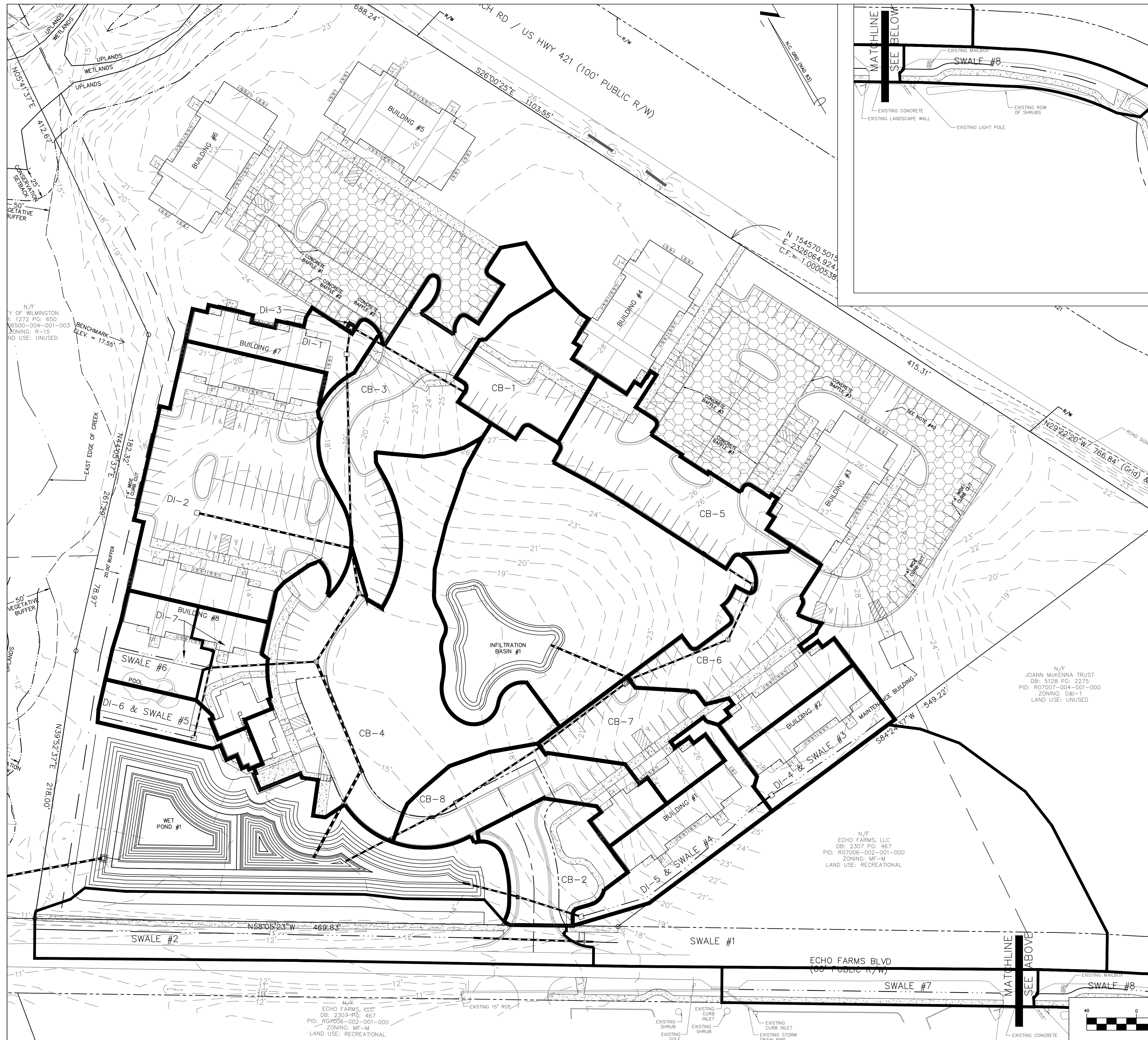
DRAINAGE AREA MAP—INLETS & SWALES SCALE: 1"=40'
